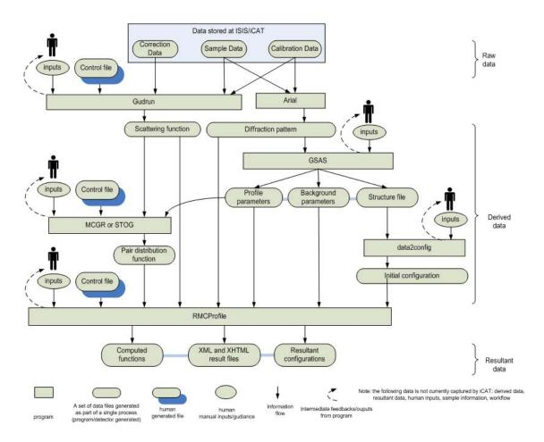
Figure 4: Cambridge Earth Sciences Crystallography Workflow [30]
