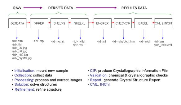
Figure 3: EPSRC NCS Crystallography Workflow
